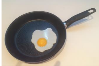
Light hearted example Adhering a 3d printed PU to a "non-stick" surface with an LSE bonder, no pre treating
